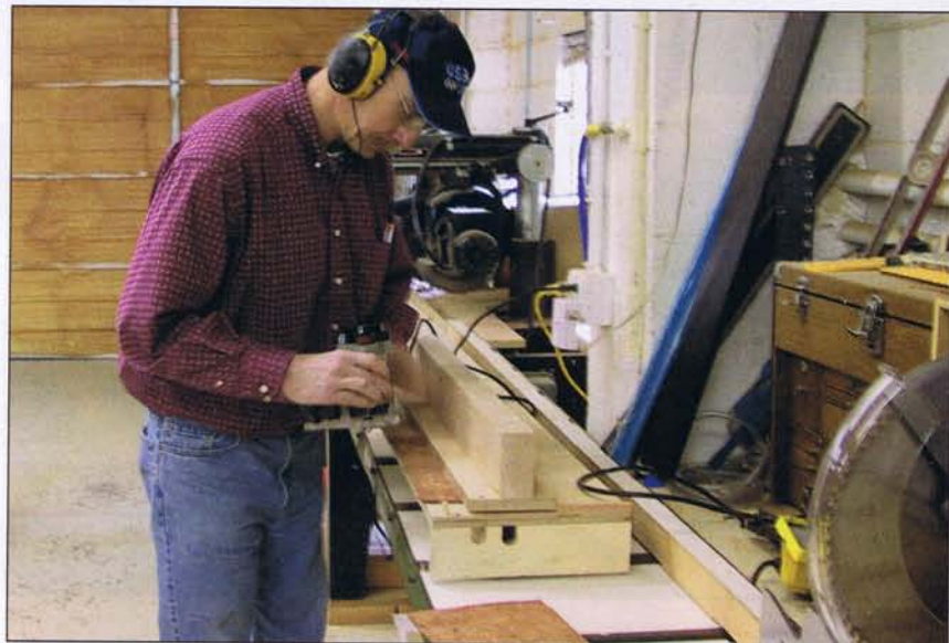
To give uniformity to the veneer he's using, Spomer takes a router to the edge of the veneer to make all the pieces even.
