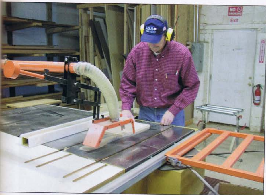
Most of Spomer's jobs begin by cutting large sheets of MDF or Baltic birch plywood on his Powermatic table saw.
