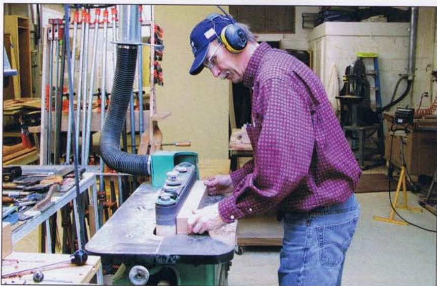
Spomer's Newton edge sander comes in handy here as he sands the leg of a side table that will resemble a Stickley piece when finished.
